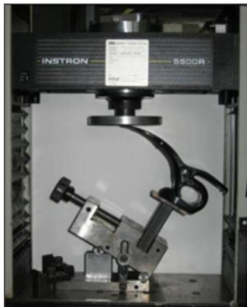
Testing for material characterization, biomechanical evaluations, and overall durability has factored strongly into the development of the foot. Much of the materials characterization testing was performed using Instron® static and dynamic testers at DuPont research laboratories.
